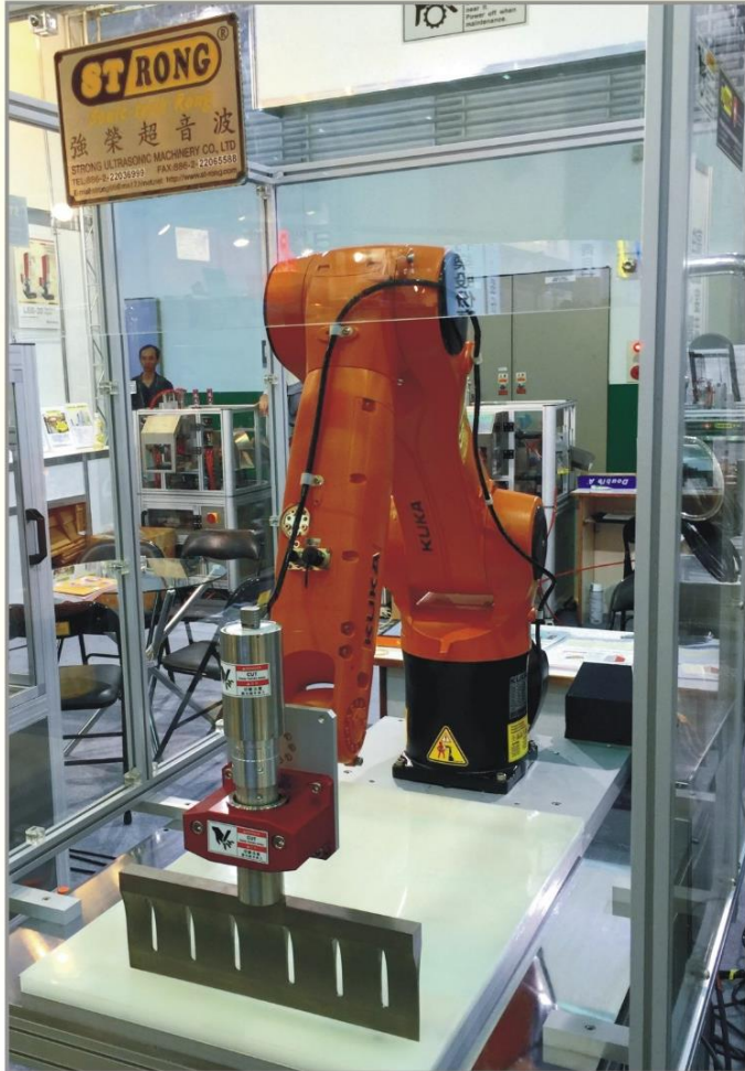
ROBOT ULTRASONIC FOOD CUTTER SRC-88
